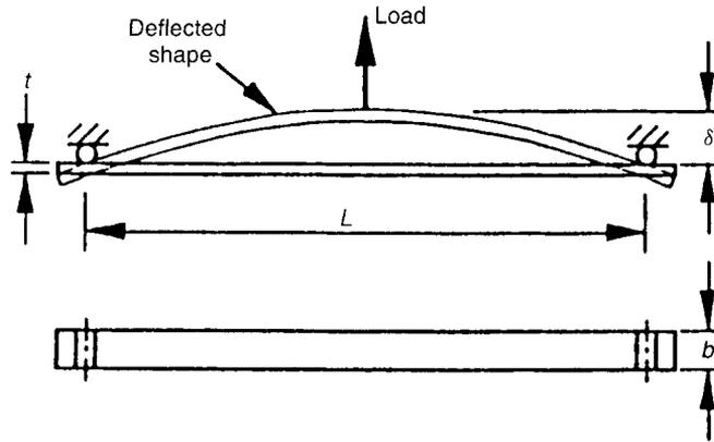
**Fig. D3.5** A truck spring. It must have a given stiffness,  $S$ , and be capable of deflection through  $\delta_{max}$  without failure. The objective is to minimize the mass  $m$ .
