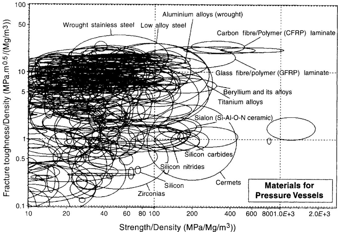
**Fig. D4.1** Part of a computer-generated Selection Chart for specific fracture toughness,  $K_{Ic}/\rho$  and specific strength,  $\sigma_f/\rho$ .
